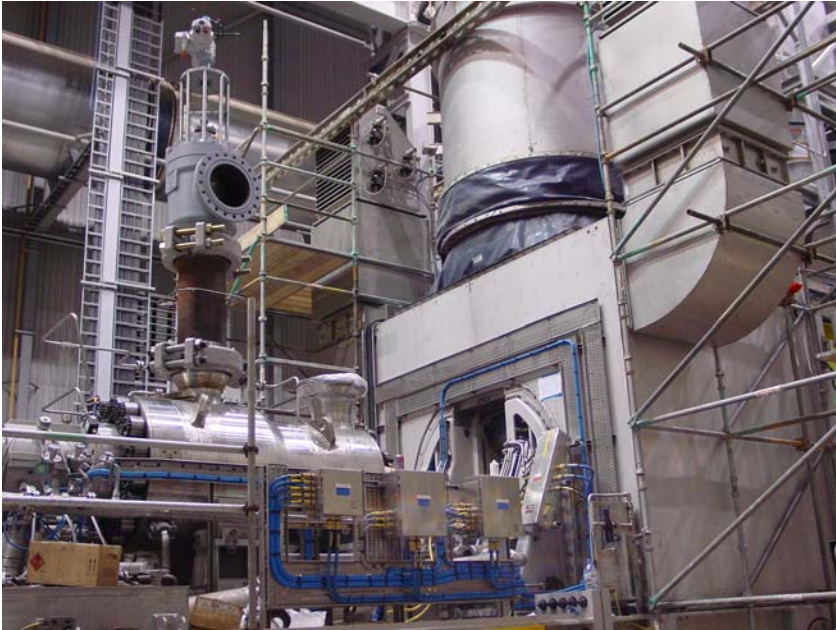
Figure 7.26 27 MW gas turbine for injection pump drive. The complete set on the test bed in Leeds/UK
